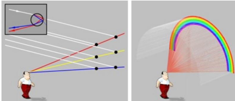
Consider now the diagram on the right which explains why the colors of a rainbow form an arc. The angle between the incoming rays of sunlight (white) and all of the red lines, forming a circular cone, have the same angle. As a result, the light that reaches your eye along these lines have the same wavelength (color). The same is true for each band of the rainbow.
