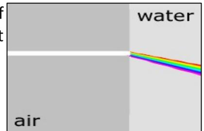
When a ray of sunlight enters a raindrop, it bends (refracts). The light then strikes the back of the raindrop, where some of the light passes through and some is reflected. As the light exits the raindrop, it is refracted again. The angle at which the light emerges depends on the wavelength of light. This path is illustrated in the small box below, where only the bending of two wavelengths (blue and red) are shown.
